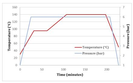
$<sup>^2</sup>$  Use  $\,$  0,2bar /min pressure ramp. Maintain a pressure of 6 bar for the entire cure cycle. Vacuum bag pressure: -0.9 bar.
